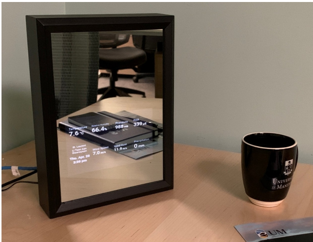
Fig. 3. Smart mirror showing weather data from MMF Weather Keeper station.
