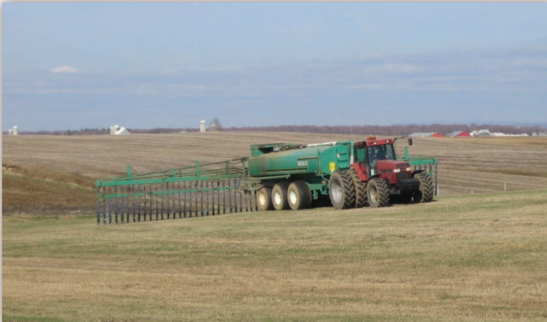
The hog slurry management BMP uses spreaders adapted with trailing hoses in order to reduce N losses to the atmosphere.
