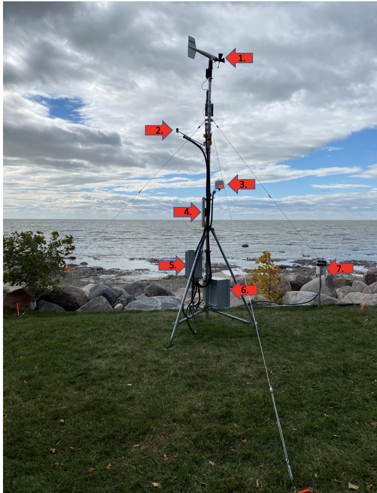
Figure 3.3: Completed Tripod with Sensors attached. (1) Anemometer (2) PAR SmartSensor (3) Temp/RH SmartSensor (4) Solar Panel (5) Logger Housing Box (6) Battery Housing Box (7) Rain Gauge
