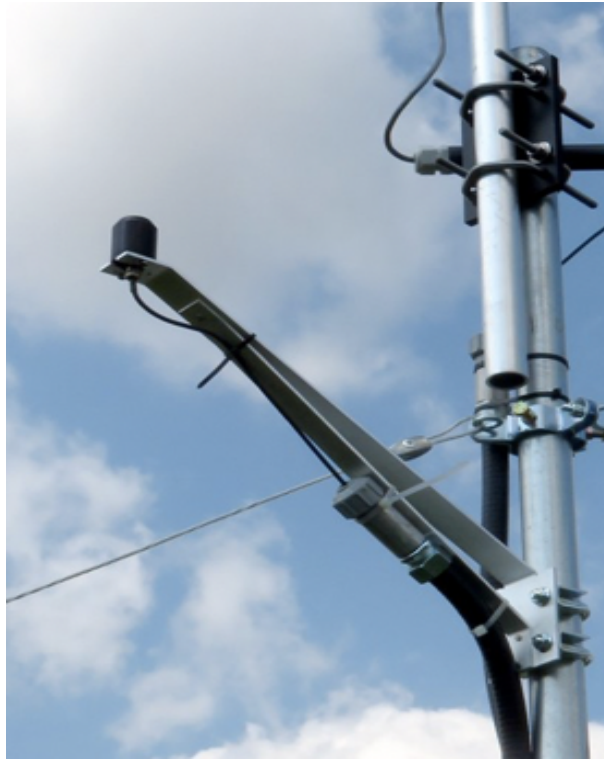
Figure 2.3: PAR sensor and mounting bracket.
