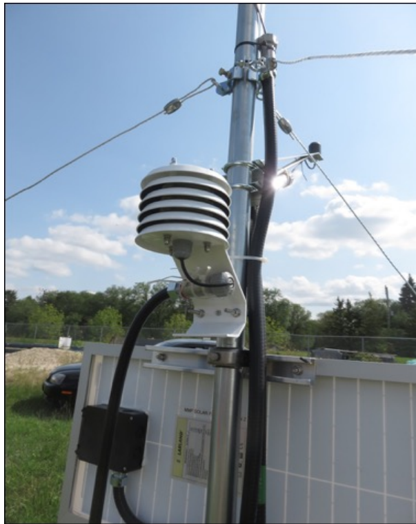
Figure 2.4: Solar radiation Shield with Smart Sensor adapter.
