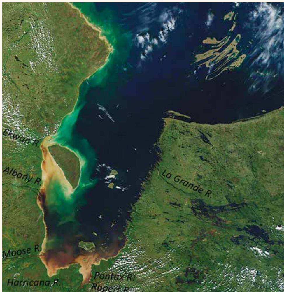
Figure 2-10. Satellite image of James Bay from August 15, 2022. The pale yellow coloured areas along the west coast are shallow mudflats. Swirling pale yellow and blue coloured features are turbid waters carrying fine-grained resuspended sediments. River discharge that appears dark brown is rich in coloured dissolved organic matter (CDOM). Several rivers are labelled.
