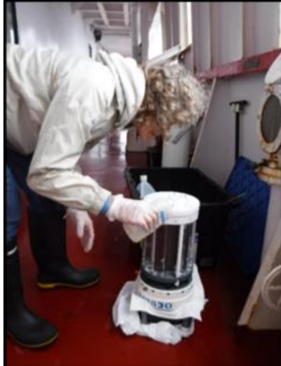
FIGURE 6.8 The rosette of the sediment traps being filed with a density gradient solution before deployment
