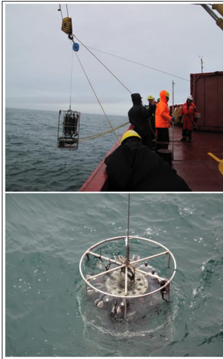
FIGURE 1.10 Rosette (10 bottle) operations on board CCGS Des Groseilliers.
