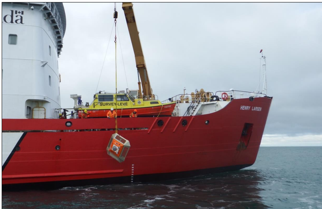
FIGURE 6.2 Lifting the TRBM (NE02) onboard Henry Larsen
