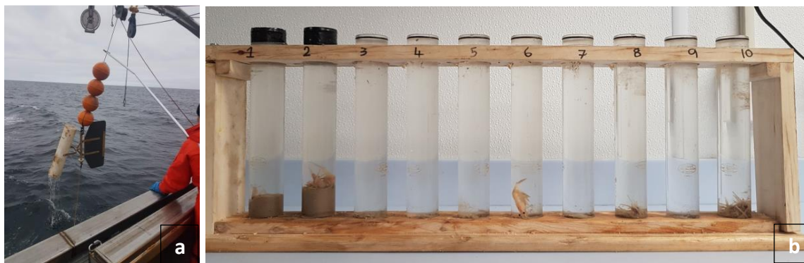
FIGURE 8.6 a) Sediment trap from mooring JB02-16 being hoisted onboard R/V William Kennedy. b) The vials from the sediment traps in the vial rack.
