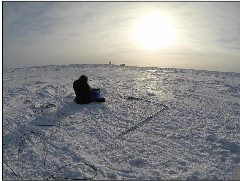
FIGURE 2.12 Preparation of under-ice light measurement through a metal arm with an attached radiometer.
