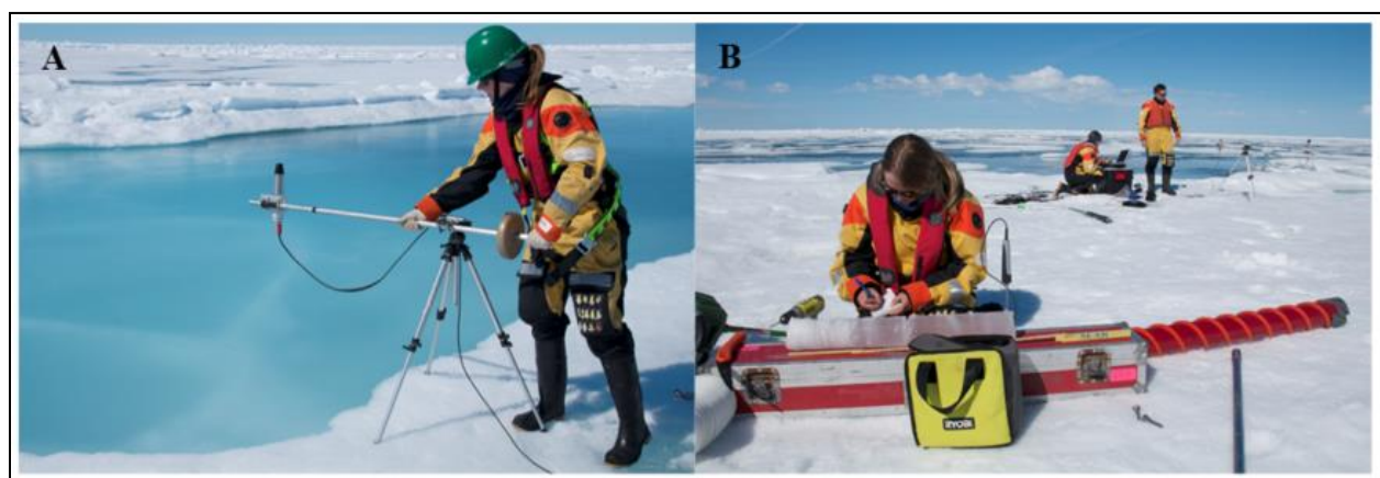
FIGURE 7.25 Measurement of surface albedo (A) and ice core sampling (B)
