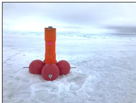
FIGURE 7.8 The surface portion of the ice-tethered mooring. There is a GPS tracker within the surface unit that allowed us to recover the unit after 6 days
