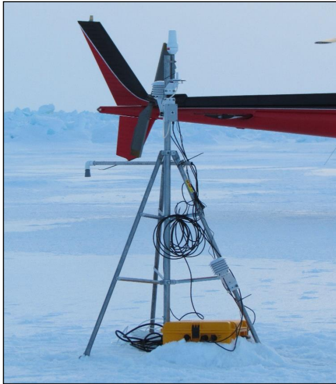
FIGURE 2.8 CEOS IMB deployed on the mobile ice. Note the yellow logger case that houses the batteries and hardware, acoustic snow sounder deployed to the left of the tower, air temperature and pressure shields at the top of the tripod and the iridium antenna at the very top.
