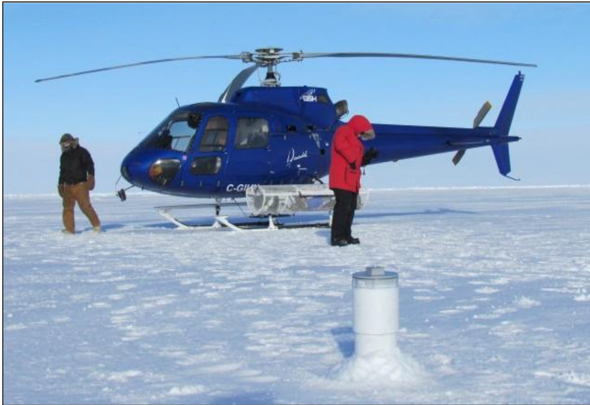
FIGURE 2.7 Ice beacon deployed on a mobile ice floe. Approximately 12" is visible above the snow.
