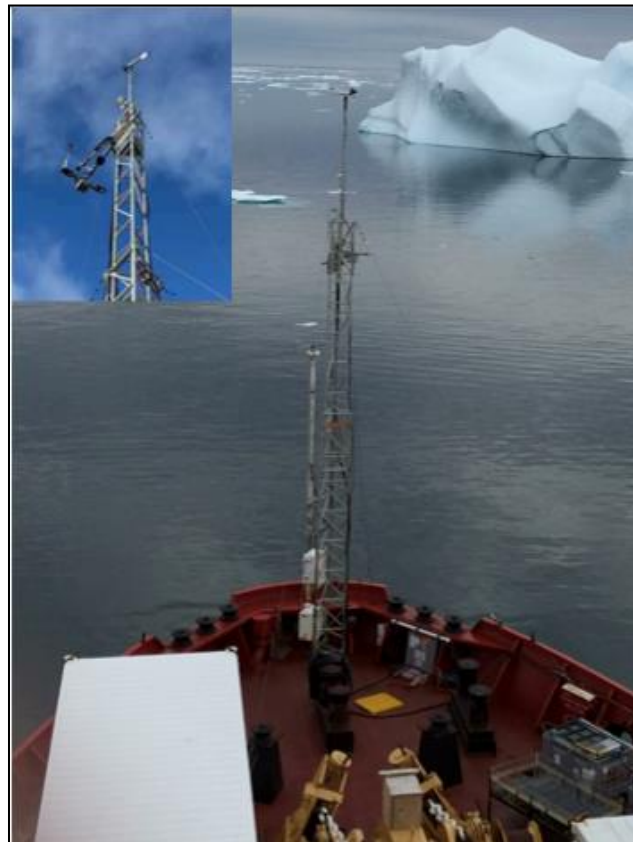
FIGURE 7.32 The metrological tower located on the foredeck of the Amundsen with EC flux system (inset)
