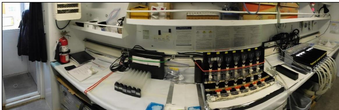
FIGURE 7.24 General set-up for the PE incubations in the Radvan. From right to left: inoculation space, incubator, filtration ramp, clean workspace (Photo Credit: Rachel Hussherr)
