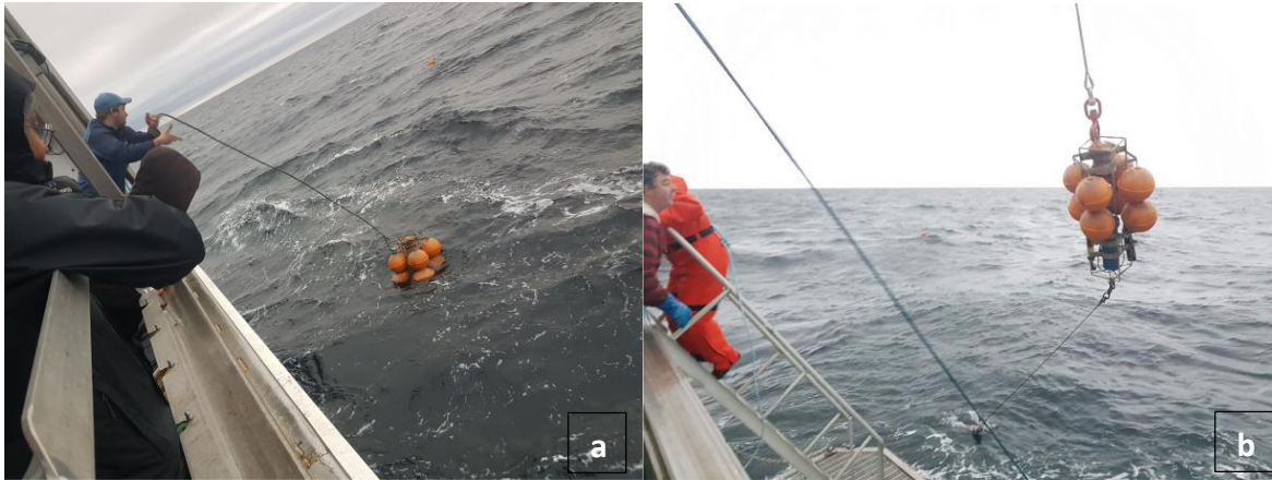
FIGURE 8.3 a) Acoustically released mooring with floats being recovered using a grapnel from R/V William Kennedy, b) Mooring being recovered using the aft winch.
