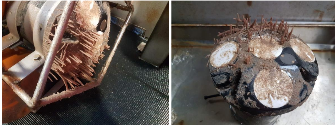
FIGURE 8.5 Biofouling of Signature 500 ADCP.
