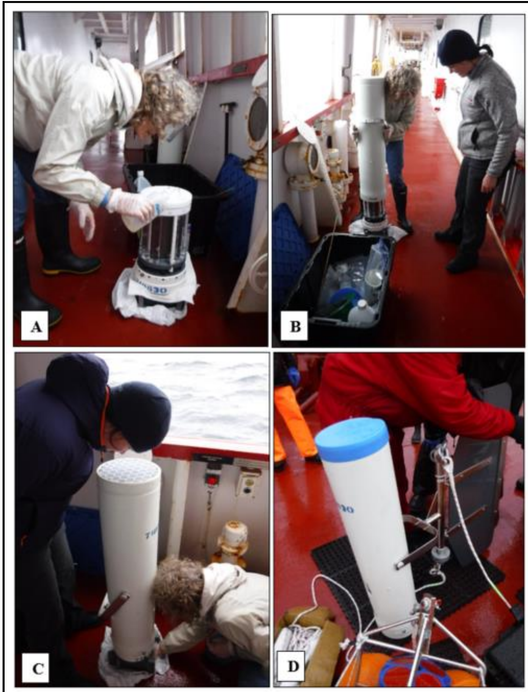
FIGURE 1.8 (A) Mary O'Brien fills sediment trap tubes with density gradient solution that are housed in a rosette assembly that also contains the motor/timer, and (B) then places and secures the corresponding PVC tube that houses an asymmetrical funnel over the sediment trap tubes. (C) Michelle Kamula and Mary O'Brien ensure the sediment trap tubes are lined up with the asymmetrical funnel and that the rosette, motor/timer smoothly rotates inside the PVC tube. (D) Before deployment, a fin is securely fastened to the sediment trap and attached to the mooring line.
