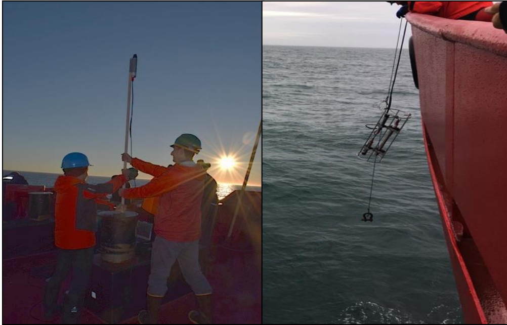
FIGURE 1.14 Measurements of incident solar radiation (left, radiometer attached to a stick pointing upward), total underwater irradiance and hyperspectral absorption and transmission within the water column (right, radiometers mounted to a metal frame and lowered with a weight a straight alignment).
