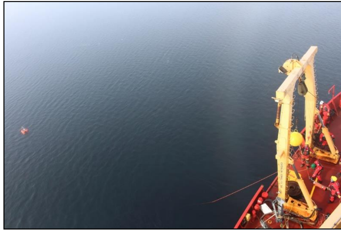
FIGURE 7.19 Anchor last mooring deployment from the foredeck
