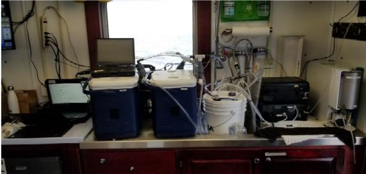
Figure 24. Algal Online Analyser and automatic incubator set up on the flow-through system where it discharges in the lab. (Photo credit: David Capelle)
