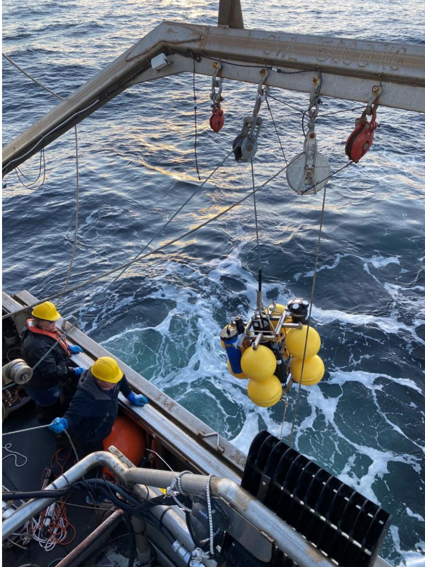
Figure 18. Mooring deployment from the stern of the William Kennedy using the A-frame.
