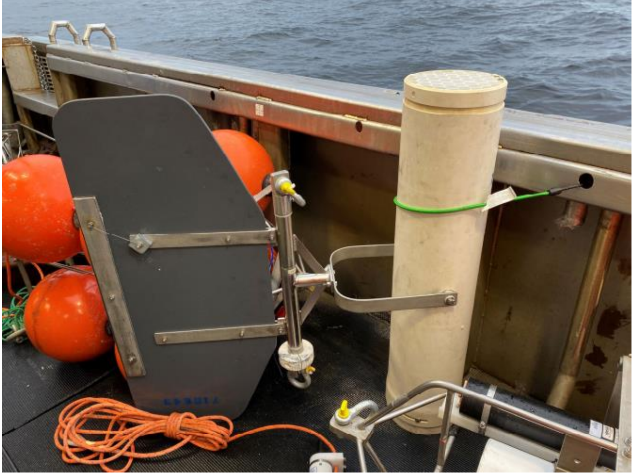
Figure 16. Baker-style sediment trap by Gurney Instruments, assembled on stern deck prior to deployment.
