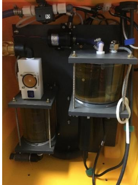
Figure 35 The underway optode / GTD (PIGI) system installed in the forward lab
