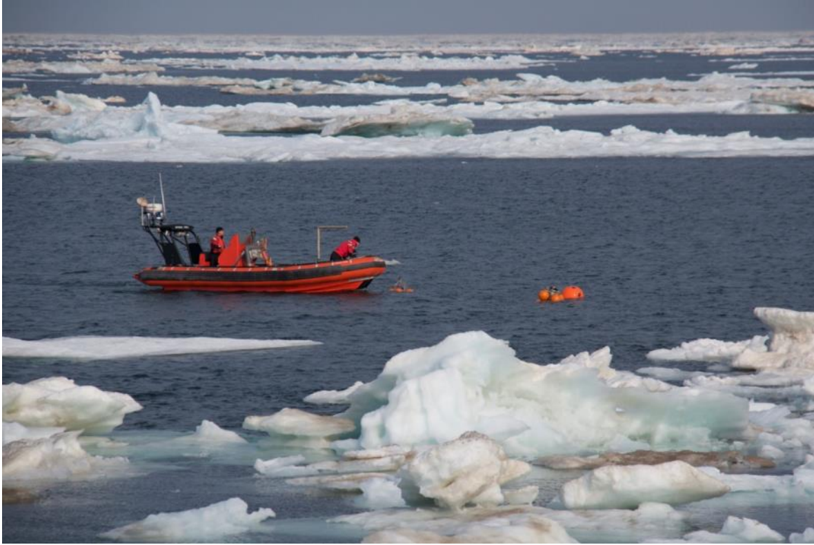
Figure 14 Mooring recovery with an assistance of zodiac
