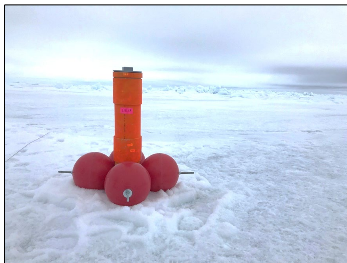
Figure 8 The surface portion of the ice-tethered mooring. There is a GPS tracker within the surface unit that allowed us to recover the unit after 6 days
