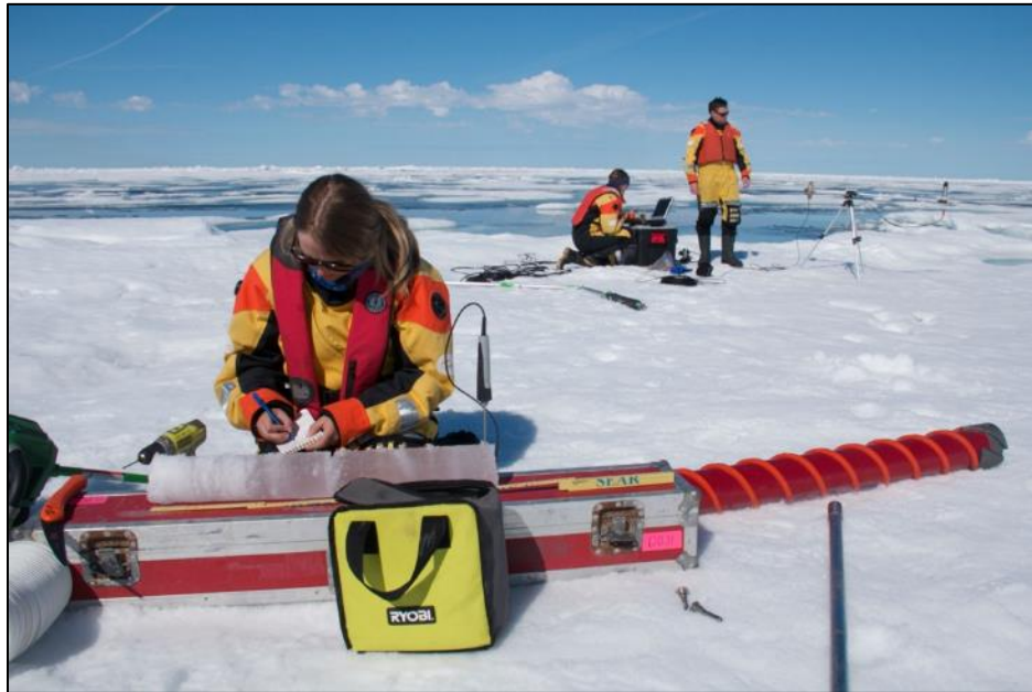
Figure 5 Laura Dalman measuring the ice temperature profile of an ice core
