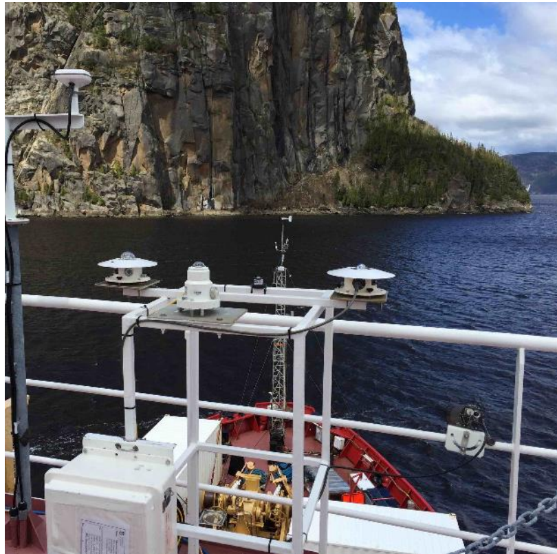
Figure 31 The radiation sensors and digital camera located above the wheelhouse of the Amundsen. Shown are the pyrgeometer (right), pyranometer (left) and PAR sensor (centre back) and UV sensor (centre front). The automated digital camera is mounted on the rail below and to the right of the pyrgeometer.
