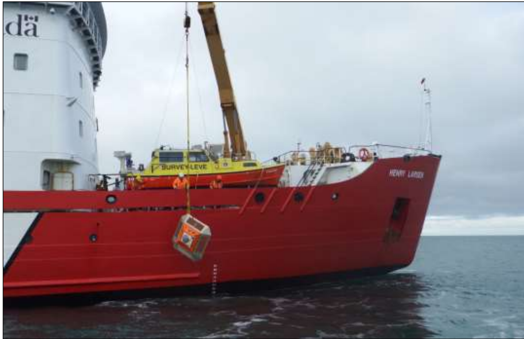
Figure 3. Lifting the TRBM (NE02) onboard Henry Larsen.
