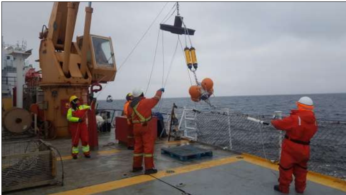
Figure 6. Mooring deployment from the helicopter deck
