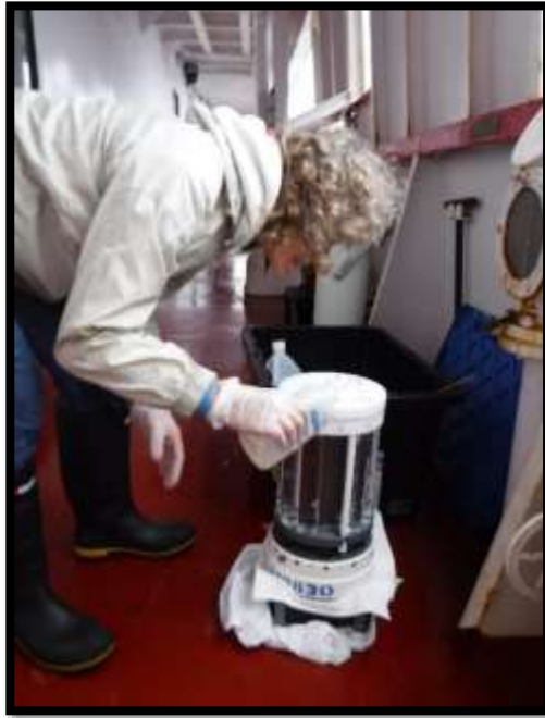
Figure 9: The rosette of the sediment traps being filled with density gradient solution before deployment.
