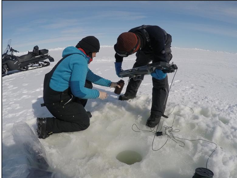
Figure 12 Water sampling using a niskin bottle
