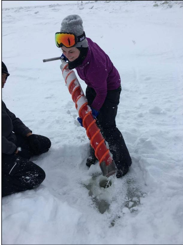
Figure 11 Pulling up the core barrel after taking a full ice core
