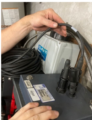
Figure 16. pCO 2 system attached to the flow-through system, which brings in seawater through the ship's hull from a depth of about 2 m below the sea surface. (Photo credit: J. Hunt)
