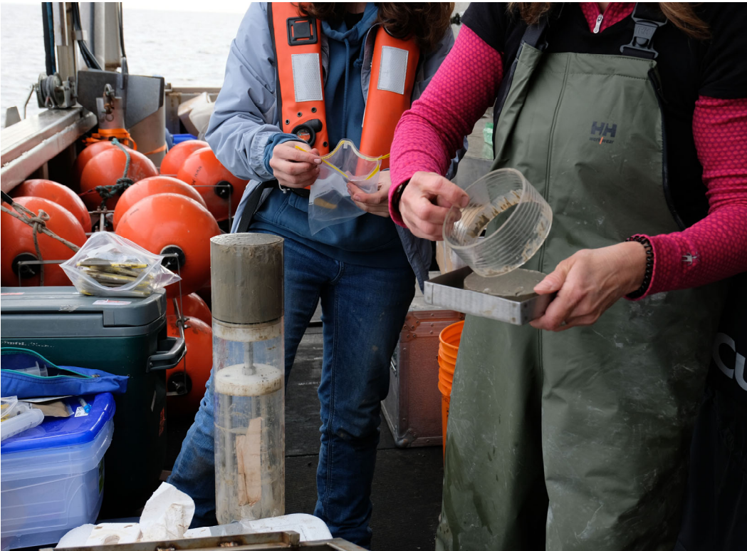
Figure 28. Extruding and sectioning a sediment core. (Photo credit: M. Durand)
