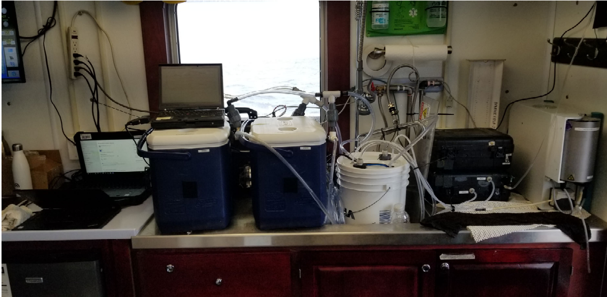
Figure 18. Algal Online Analyzer and automated incubator set up on the flow through system where it discharges in the lab. (Photo credit: D. Capelle)
