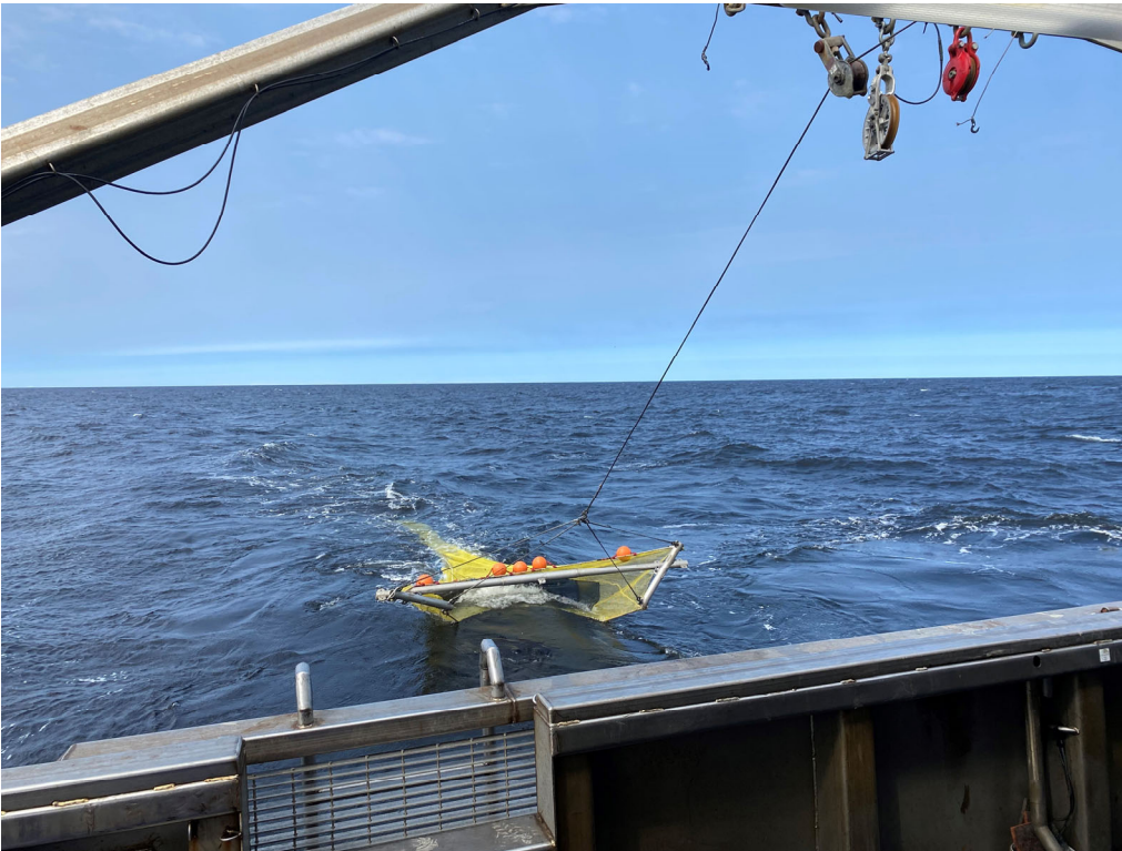
Figure 22. Benthic beam trawl being deployed over the stern.
