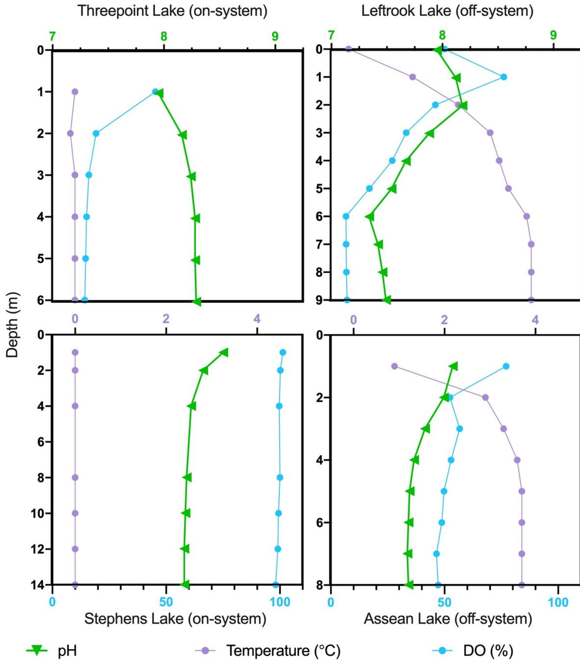
Figure 3.2b: Water quality parameters in on-system (left) and off-system (right) lakes collected from the ice surface using a Water Quality Instrument (Pro Plus, YSI) in March/April 2017.
