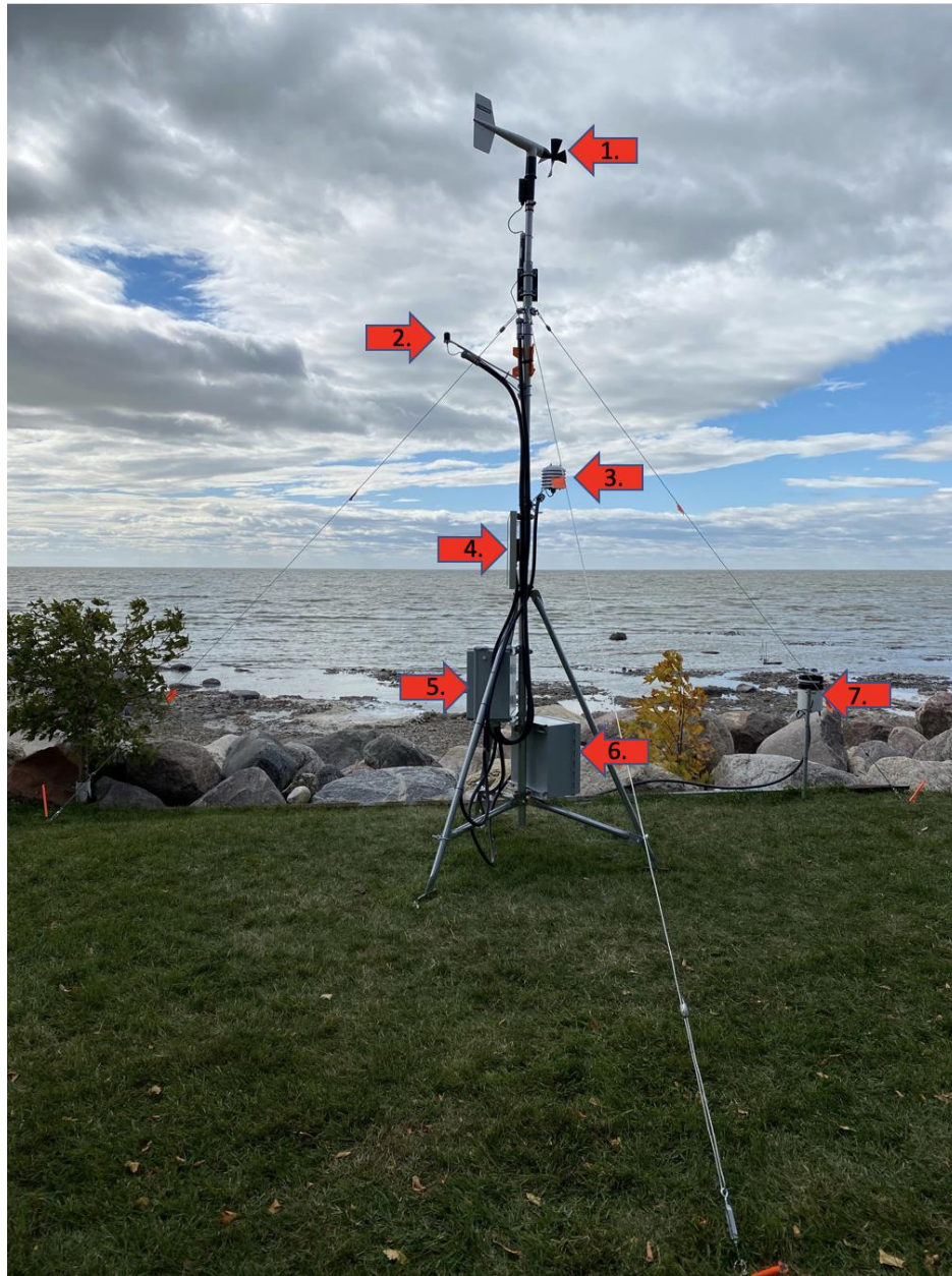
Figure 1. Complete weather station with (1) Anemometer, (2) PAR sensor, (3) Temperature and relative humidity, (4) solar panel, (5) logger housing box, (6) battery housing box, (7) Rain gauge or bucket, and guy wires identified with orange flagging tape.
