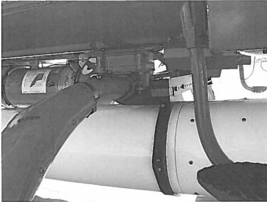
Forward mount structure, clamping ring, and slip joint (secured with #10 fasteners) between root tube and middle tube.
