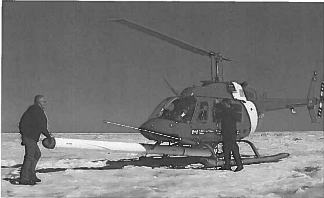
206L system installed. Note vertical cable run visible between auger and pilot Harrison Macrae.
