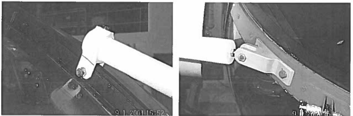
Figure 4: Photographs 4 and 5: mounting strut connection to central rib (left) and port mounting strut ball-end mounted in stanchion (right). Care should be taken to adjust ball-ends such that sensor roll reading is zero when helicopter is on a level surface.
