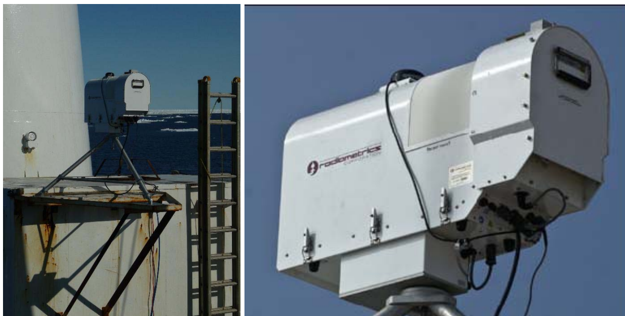
Figure 69: TP/WVP 3000A mounted on the roof of the CCGS Amundsen ‘met shack.’
