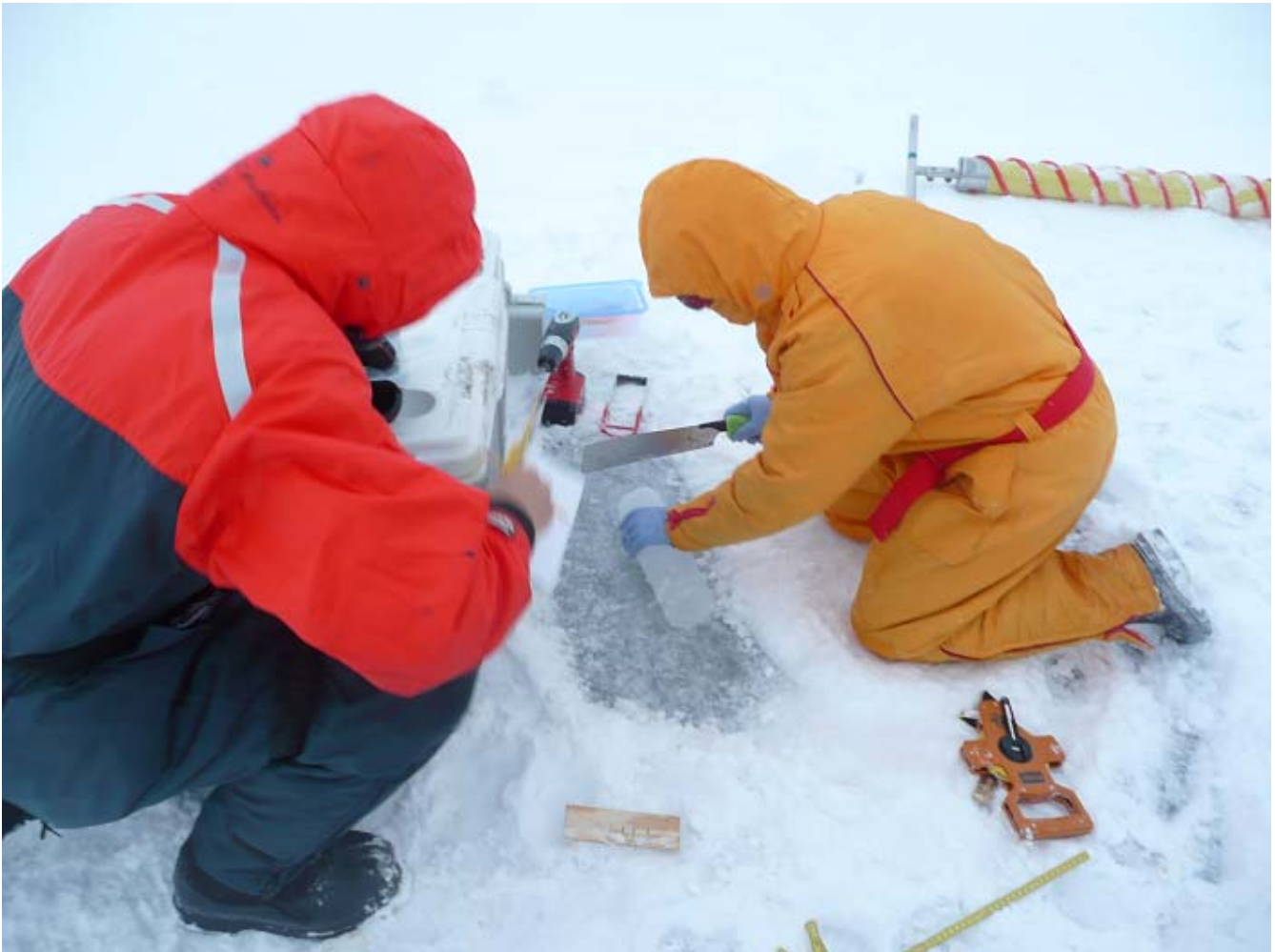
Figure 55: An ice core being cut into 10cm segments for eventual salinity analysis
