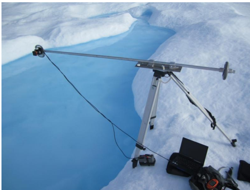
Figure 62. The laser profilometer mounted over a melt pond.
