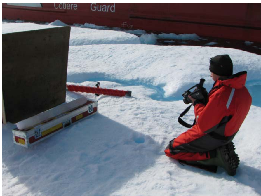
Figure 57. Taking IR image of an ice core, Aug. 17, 2011
