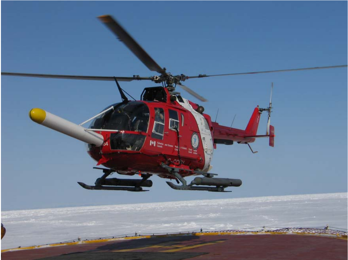
Figure 15. Canadian Coast Guard helicopter showing the fix-mounted sensor equipment.
