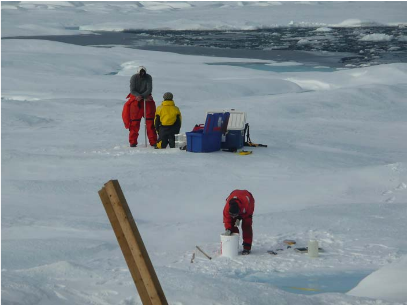
Figure 54: On-ice team taking an ice core for temperature and salinity profiles (top left), and sampling area, depth, temperature and salinity of meltponds (lower right).
