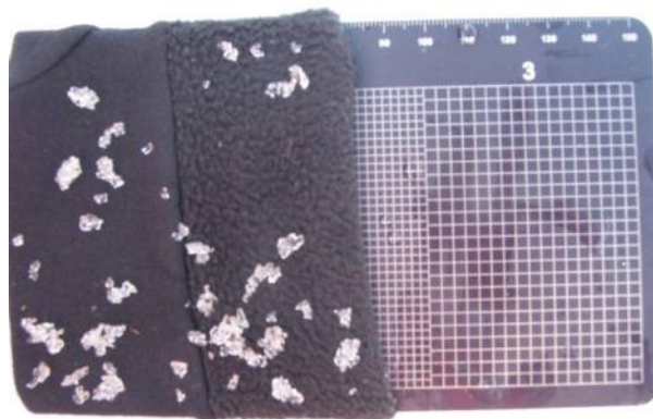
Figure 61. Example surface granular layer photograph. Grains were placed on a felt insulator next to the grid as they would melt when placed directly on the metallic grid surface.
