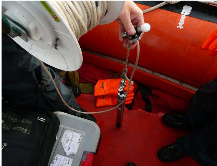
Figure 9. An Idronaut Ocean Seven 304 CTD-T probe about to be deployed.
