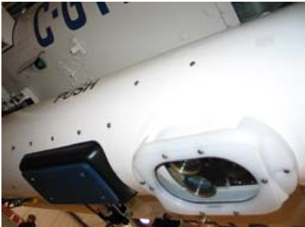
Figure 16. Sensors and Software Noggin 1000-NIC GPR System (left) protruding from section of the mounting tube of a 206L helicopter along with laser/video camera (right).
