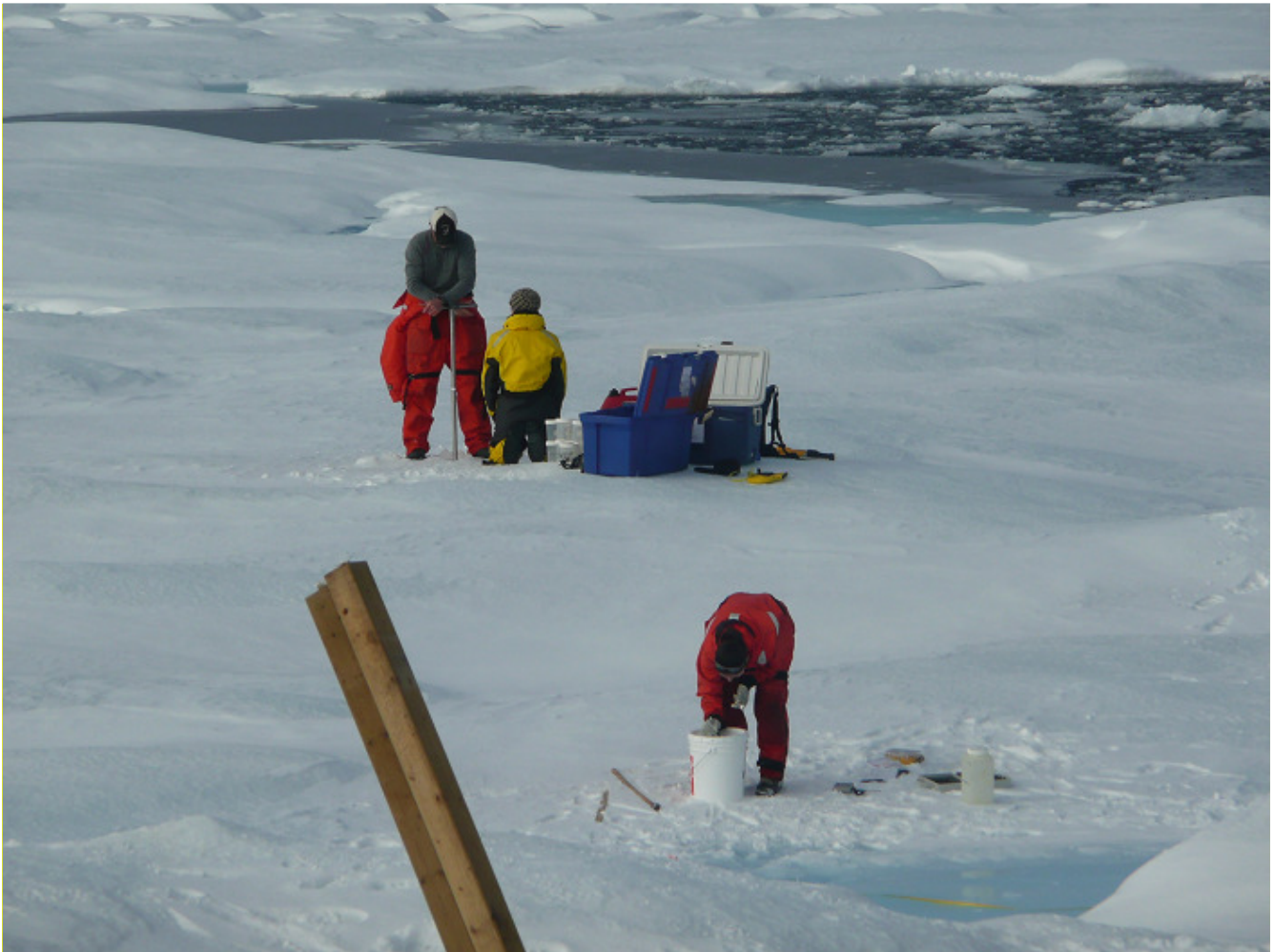
Figure 17: On-ice team taking an ice core for temperature and salinity profiles.
