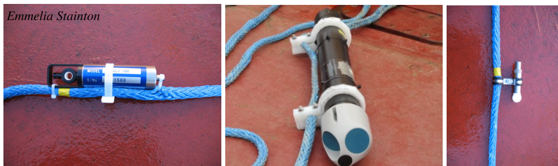
Figure 12: Mixed-Layer buoy subsurface instrumentation. [Left] JFE ALEC ® compact CT sensor. [Middle] Aquadopp current profiler. [Right] JFE ALEC ® PAR sensor.
