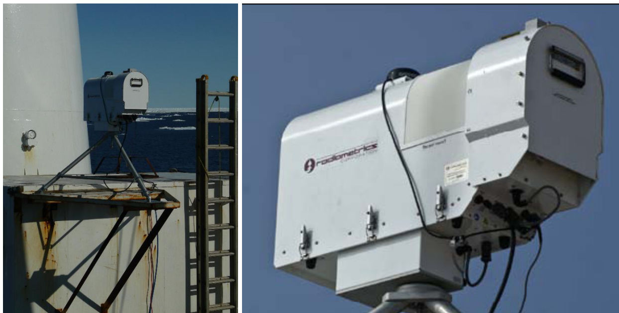
Figure 28: TP/WVP 3000A mounted on the roof of the CCGS Amundsen ‘met shack.’
