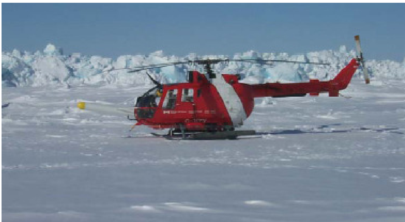
Figure 13: The IcePic, a fix-mounted helicopter-borne electromagnetic is shown mounted on a BO105 CCG helicopter. The red pod fixed to the helicopter skid-gear houses the video and the second laser.
