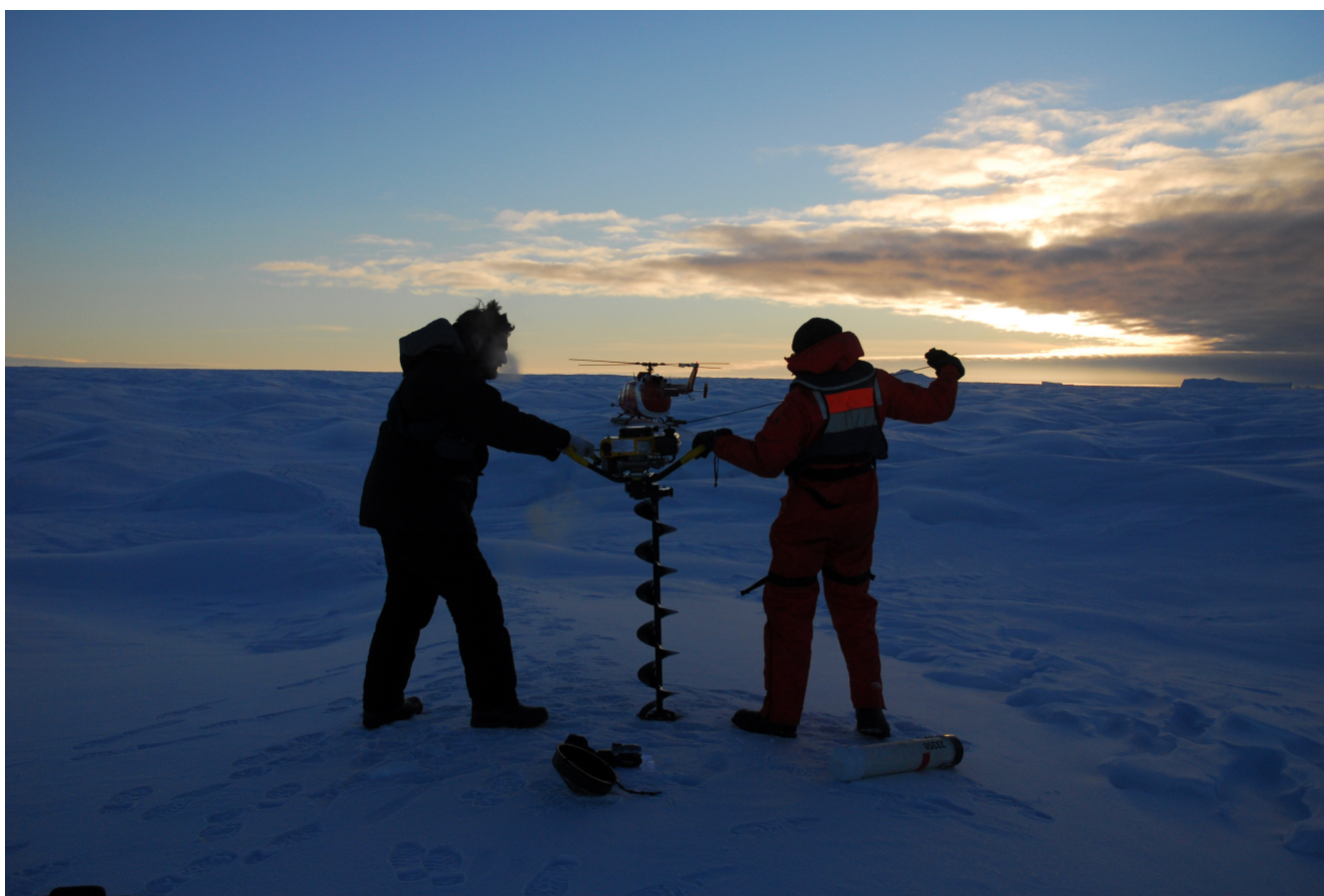
Figure 22: Ice beacon deployment. A site is selected with good line-of-sight to the horizon, and an 8" 20-cm deep hole is drilled using a gas-powered auger. The beacon is installed upright, and activated.
