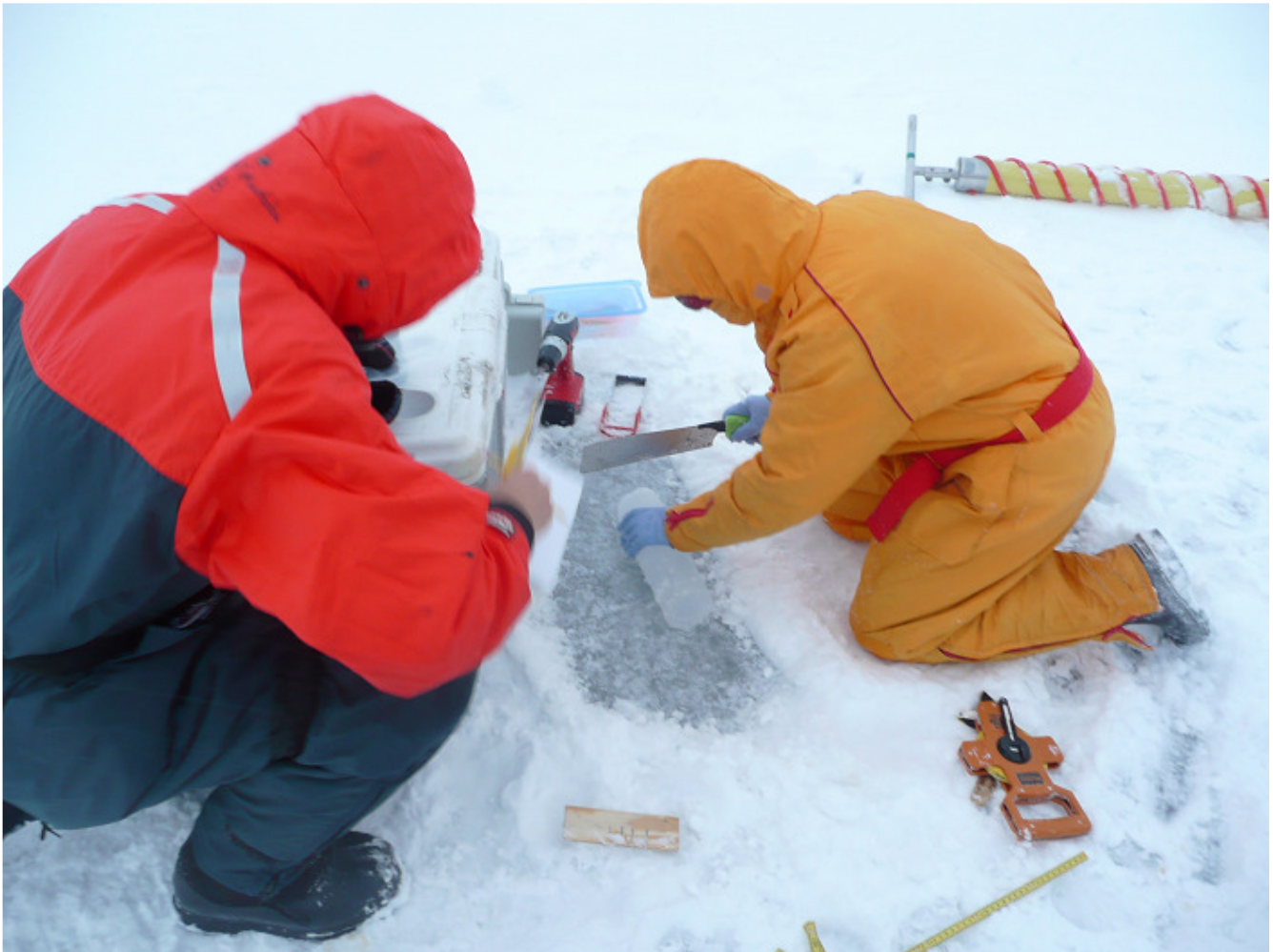
Figure 18: An ice core being cut into 10cm segments for eventual salinity analysis
