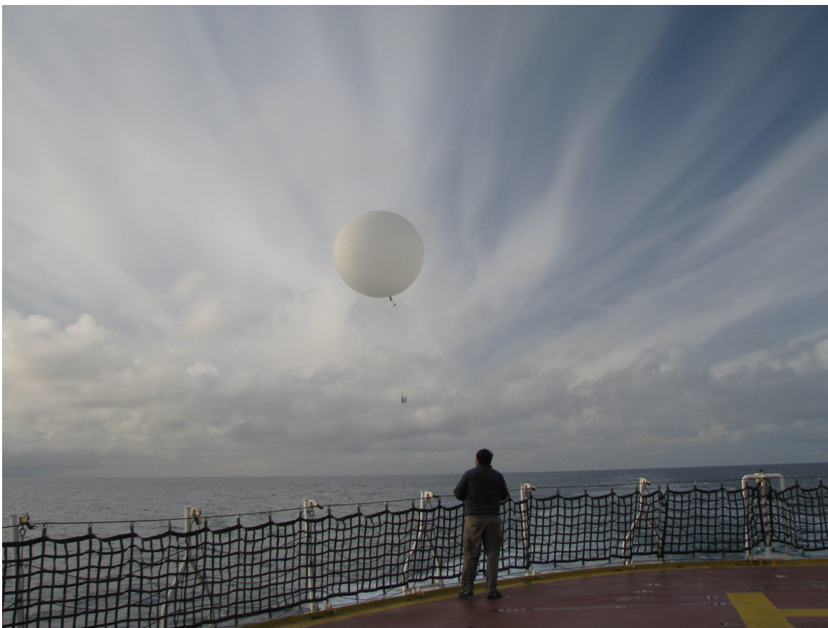
Figure 30: A weather balloon with attached radiosonde, launched from the helicopter deck.
