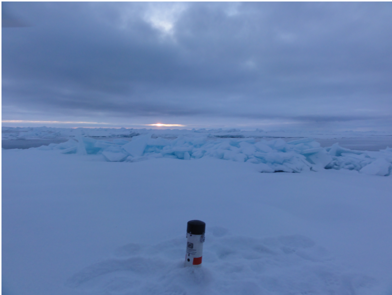
Figure 21: An Oceanetics model 703 Iridium Ice tracking buoy. The number on the front corresponds to the last five (sometimes six) digits of the iridium model ID.
