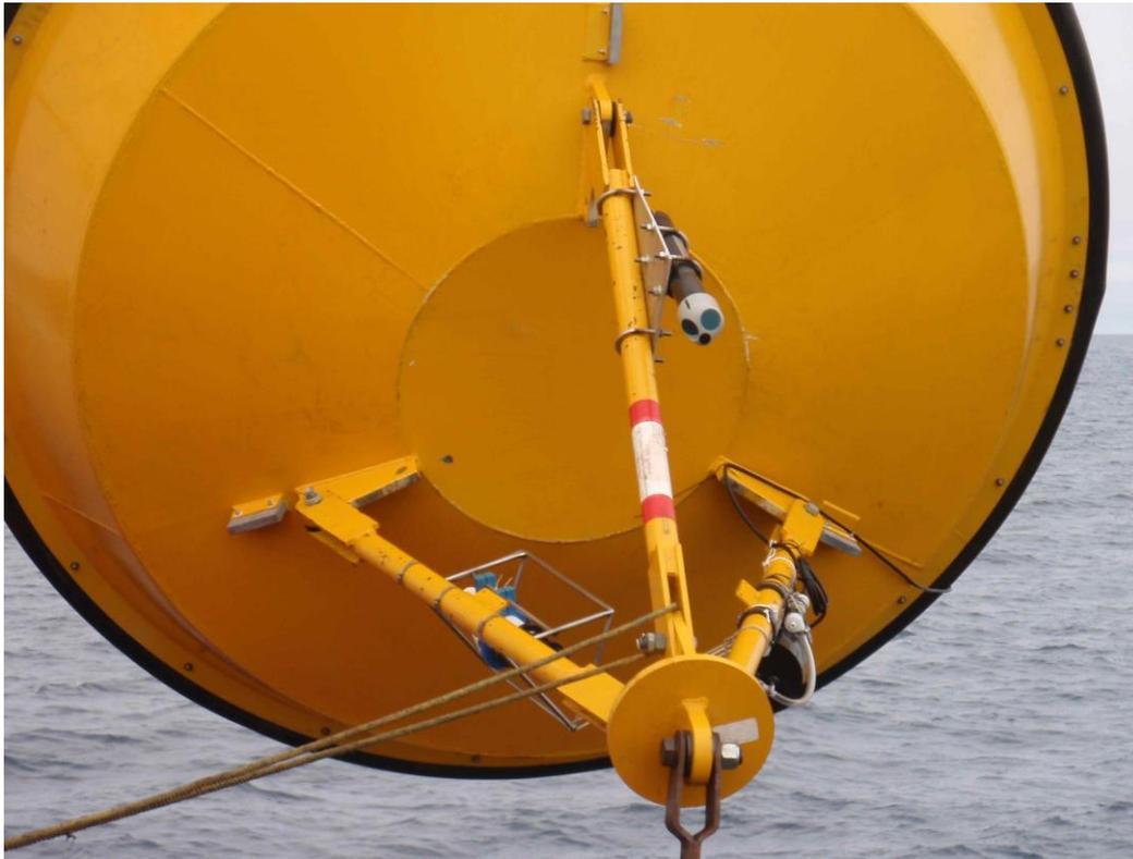
**Figure 19:** Underwater instrumentation associated with the Met/Ocean buoy. Upper panel, left to right: Nortek® Aquadopp surface current meter, RBR® multi-probe, and Pro-Oceanus® pCO<sub>2</sub>-pro. Lower Panel: installation on anchor yoke. Sensor specifics appear in Table 5. (Photos by E. Stainton and IOL consultant).
