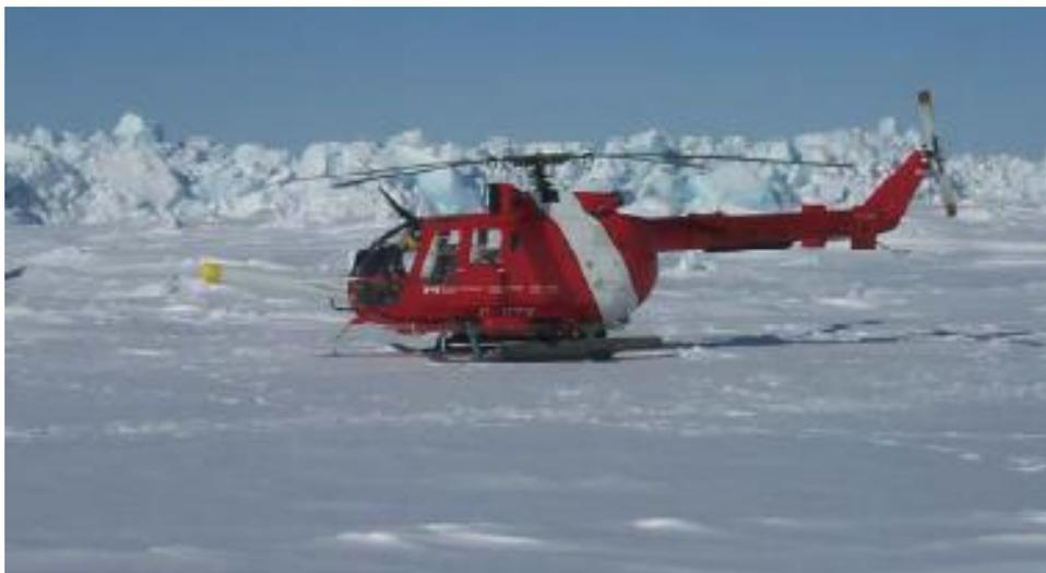
**Figure 34:** The Ice Pic, a fix-mounted helicopter-borne electromagnetic is shown mounted on a BO105 CCG helicopter. The red pod fixed to the helicopter skid-gear houses the video and the second laser.
