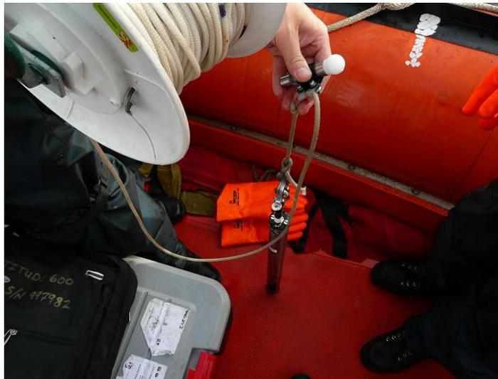
**Figure 29:** An Idronaut Ocean Seven 304 CTD-T probe about to be deployed.
