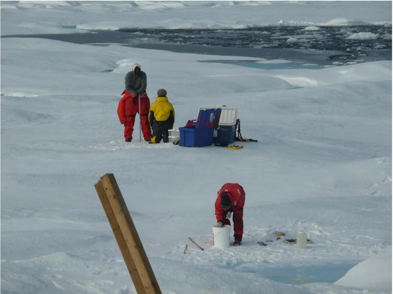
**Figure 41:** On-ice team taking an ice core for temperature and salinity profiles (top left), and sampling area, depth, temperature and salinity of meltponds (lower right).
