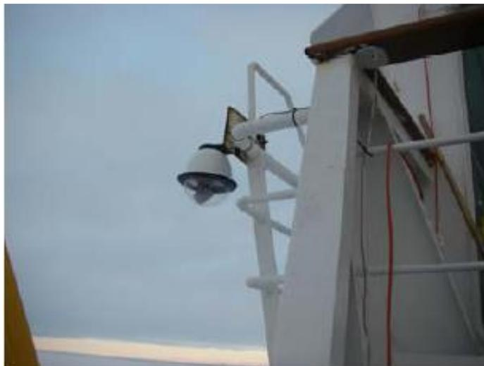
**Figure 51:** *Obliquely-mounted Canon VB-C10R mounted on the port-side railing, immediately behind the wheelhouse, and above the SBR.*
