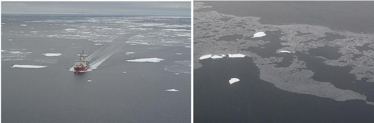
Figure 1. Ice within the northern portion of the Ajurak Block (Oct 2), a) Ice streamer from the pack ice (SIC <30%) , b) pancake ice formation (dark grey) and isolated second year ice (white).
