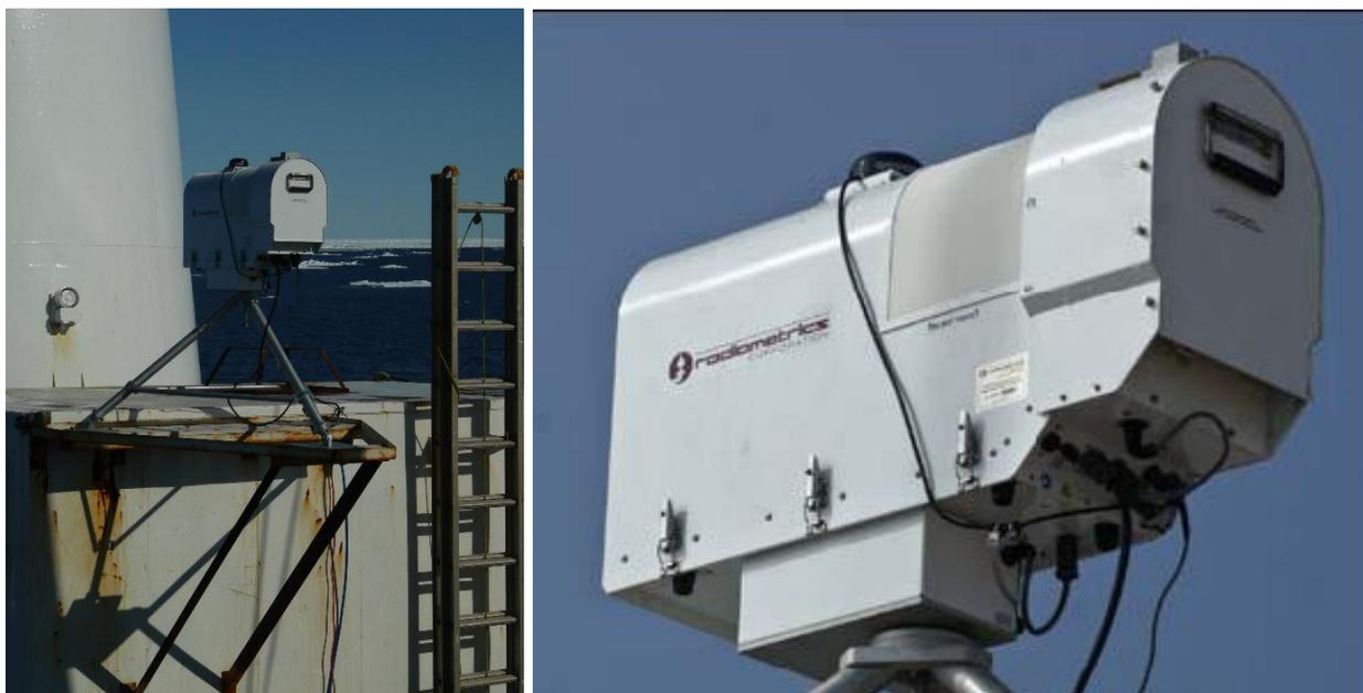
**Figure 54:** TP/WVP 3000A mounted on the roof of the CCGS Amundsen ‘met shack.’
