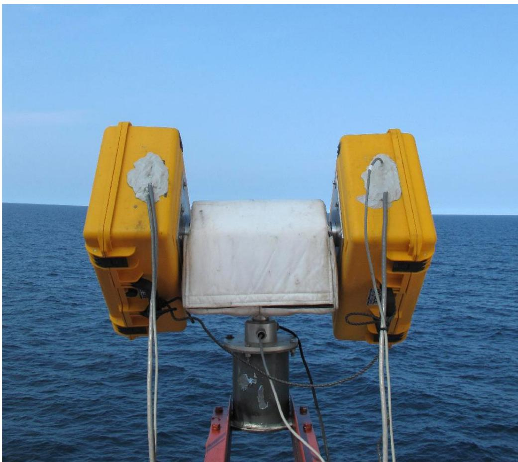
**Figure 40:** Surface based radiometer (SBR) (37 and 89 GHz) installed on port side  $\sim 10$ m above sea level.
