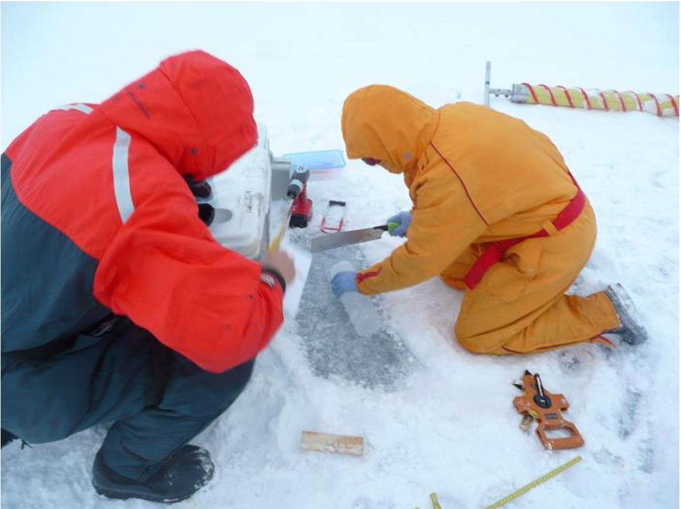
**Figure 42:** An ice core being cut into 10cm segments for eventual salinity analysis
