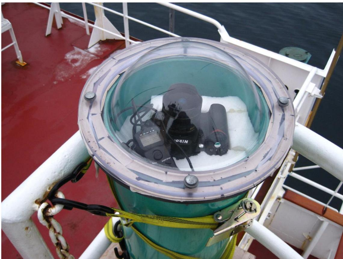
**Figure 61:** Nikon D-90 Camera with fisheye lenses attached in a weatherproof enclosure.
