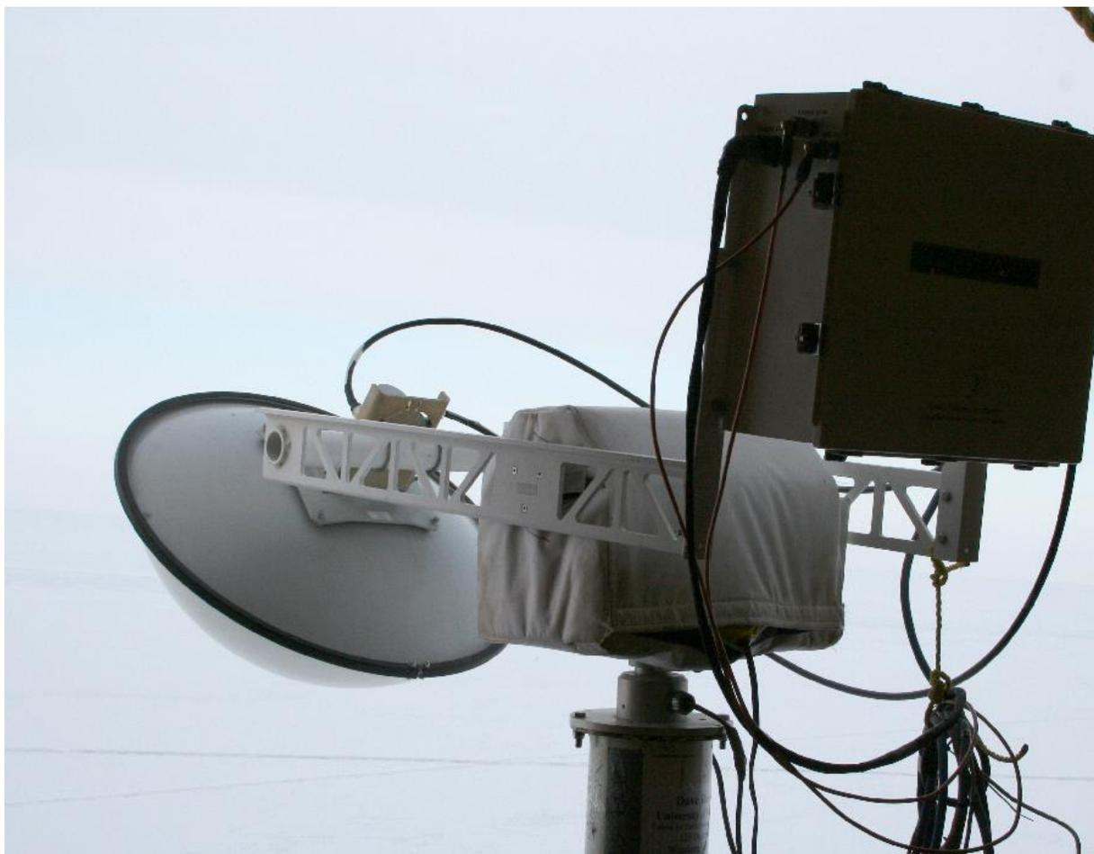
**Figure 38:** C-Band scatterometer
