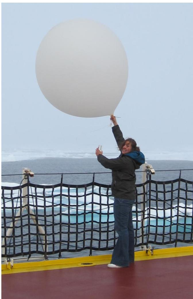
**Figure 56:** A weather balloon with attached radiosonde, ready to be launched from the helicopter deck.
