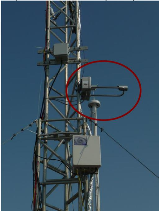
**Figure 60:** Laser precipitation gauge mounted on the CEOS Meteorological Tower.
