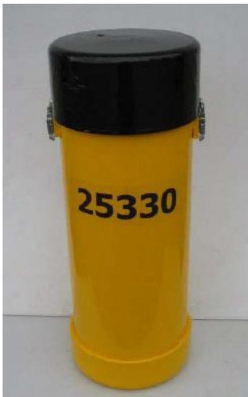
**Figure 46:** An Oceanetics model 703 Iridium Ice tracking buoy. The number on the front corresponds to the last five (sometimes six) digits of the Iridium model ID.
