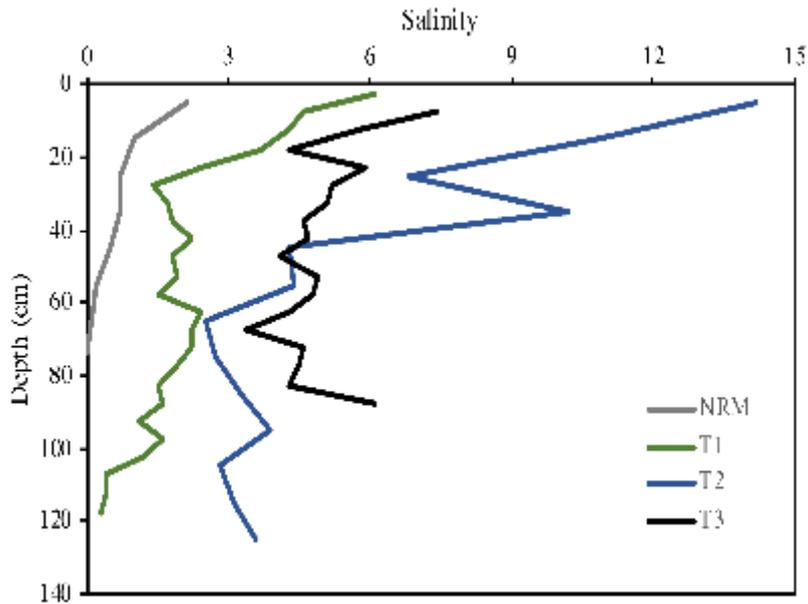
Sea ice salinity profiles from 4 locations on the landfast ice cover collected during Leg 3 (April). NRM is the Nelson River Mouth. Samples were sectioned at 10 cm intervals.
