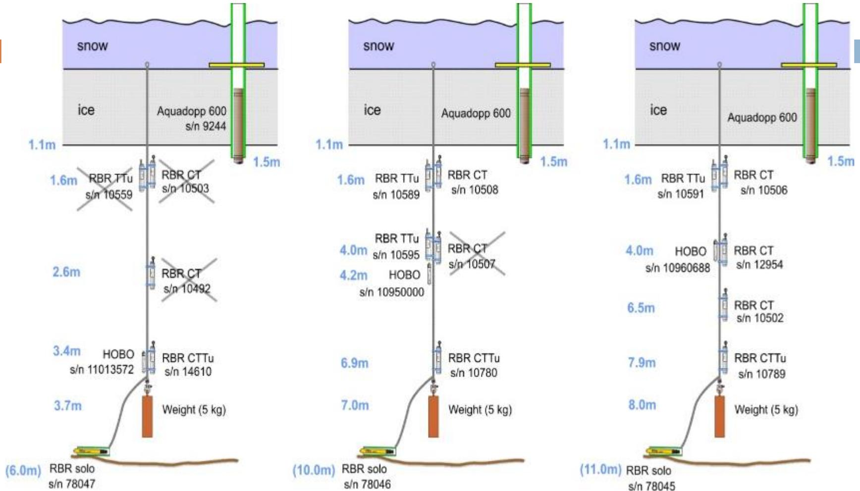
The scheme of ice-tethered moorings. The crossed out sensors indicate units that do not contain reliable records.
