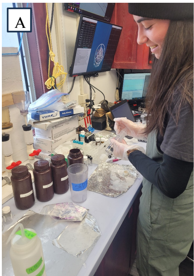
Figure 3.1. Photos of water collection and samples. (A) Kuzyk Team member C. Warnett filtering water into DOC vials (Photo credit: M. Stocking, (B) Example of a 47 mm Whatman ProWeigh® filter. Photo credit: A/B) A. Guzzi.
