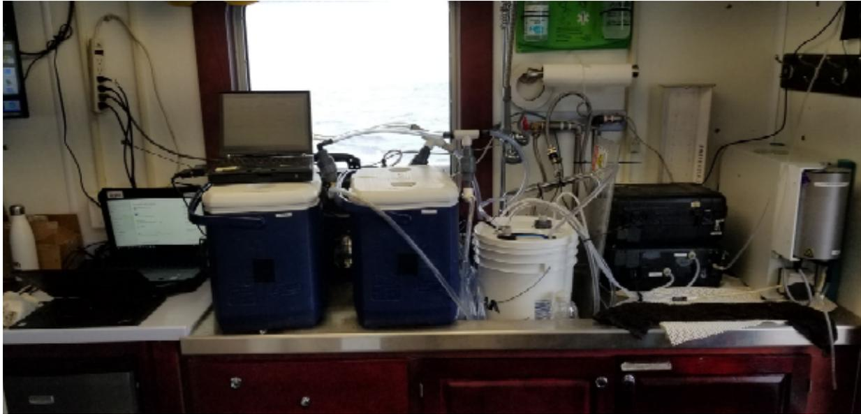
*Figure 3.4. Algal online analyzer, Dark and Light incubator chambers, and CO<sub>2</sub> sensor set up.*
