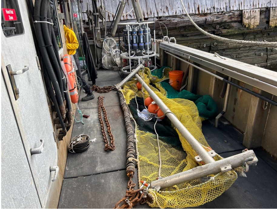
Figure 3.9 Benthic beam trawl set-up. (Photo credit: Kallie Strong DFO).
