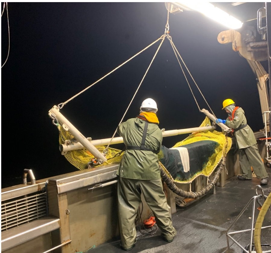
Figure 3.8. Nighttime deployment of benthic beam trawl. (Photo credit: Grace Fedirchuk CEOS).
