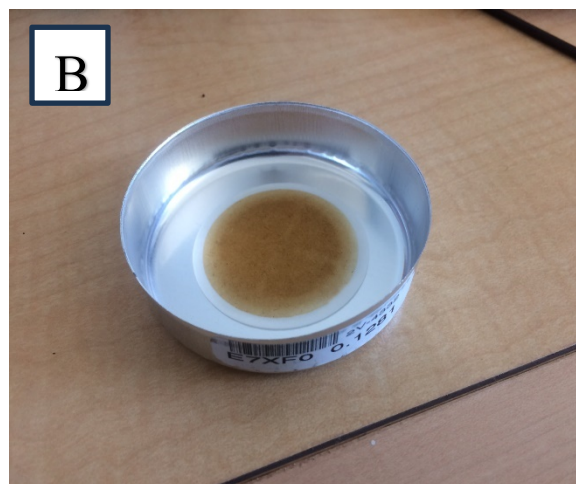
Figure 3.1. Photos of water collection and samples. (A) Kuzyk Team member C. Warnett filtering water into DOC vials (Photo credit: M. Stocking, (B) Example of a 47 mm Whatman ProWeigh® filter. Photo credit: A/B) A. Guzzi.
