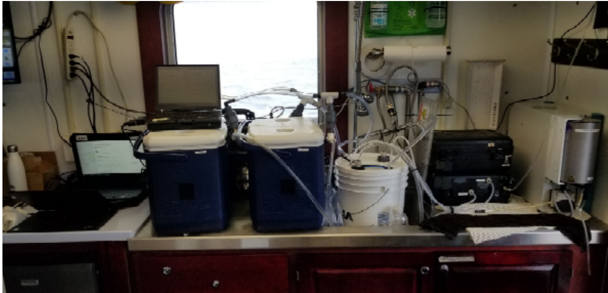
Figure 3.4. Algal online analyzer, Dark and Light incubator chambers, and CO 2 sensor set up.
